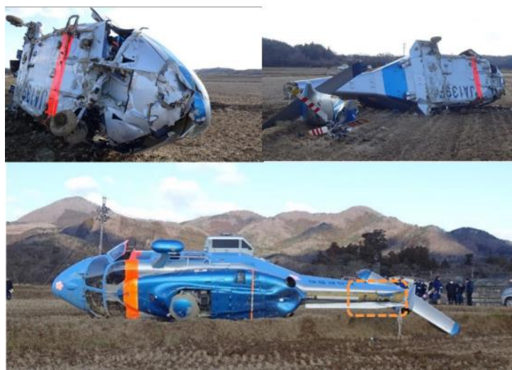
Figure 3 Rollover of the Accident Helicopter
